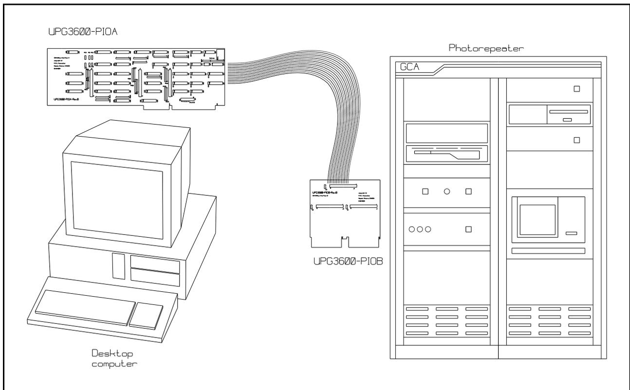
Figure B.2 : Typical UPG3696 Hardware Installation
